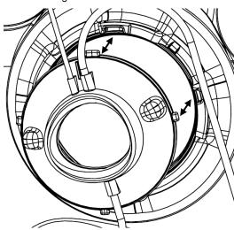
Lower the EyeSeal into the receptacle. Insert all tabs into the grooves. Grip the handles located on both sides of the EyeSeal Disposable.
