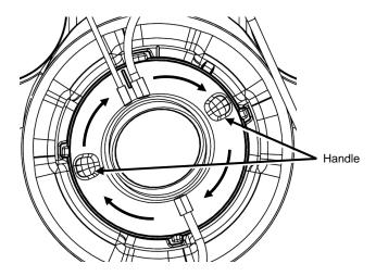
Rotate the EyeSeal Disposable clockwise until the vertical indicators are aligned.
