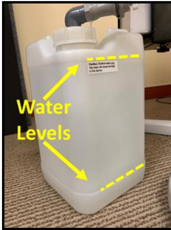
Figure 28: Water levels for Filled and Drained, respectively
