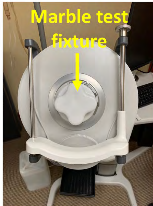
Figure 40: Marble test fixture attached to the scan head.
