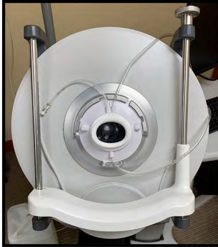
Figure 37: EyeSeal in place
