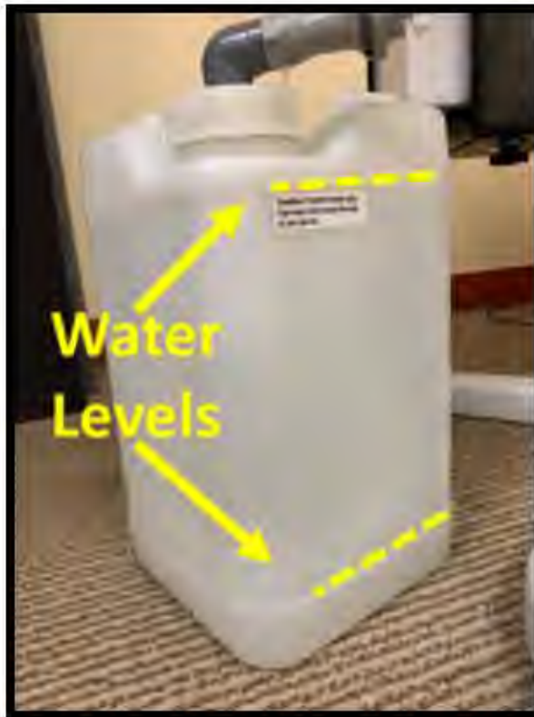
Figure 28: Water levels for Filled and Drained, respectively
